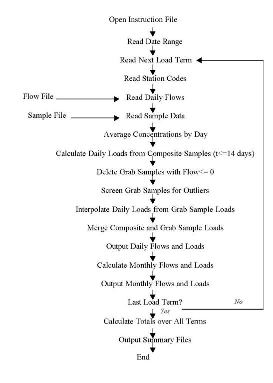
Figure B-2 Flowchart - Calculation of C-139 Basin Phosphorus Loads
