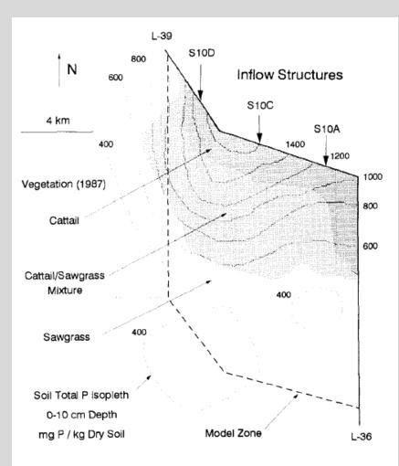
Figure 2. Cattail and Soil Phosphorus Distribution in S-10 Inflow Zone of Water Conservation Area 2A. Figure depicts boundary of model zone, gradients in vegetation (Urban *et al.*, 1993), and gradients in soil phosphorus (Reddy *et al.*, 1993; DeBusk *et al.*, 1994). Regional map is shown in Figure 1.
