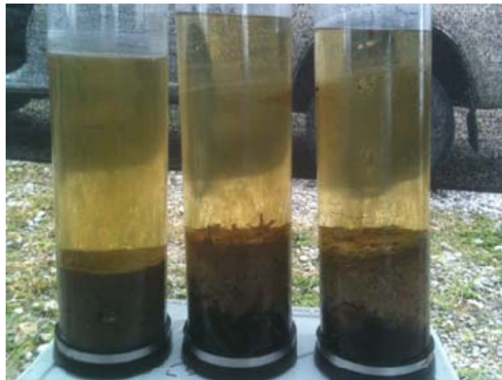
Figure 5-45. Intact sediment cores were used to examine differences in sediment P flux and enzyme activity between the PSTA cell and muck-based treatment cells in STA-3/4. Depicted are cores from the PSTA cell (left), and the adjacent SAV-dominated Cells 2B (middle) and 3B (right) (photo by the SFWMD).
