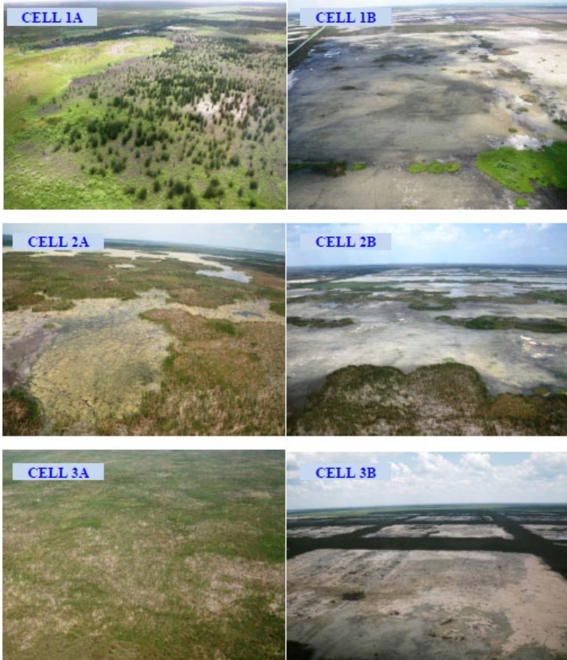
Figure 5-28. Dried out cells in STA-3/4 as a result of a regional drought, high evapotranspiration rates, seepage losses, and delayed wet season; aerial photos taken by SFWMD on June 16, 2012.
