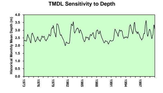
Simulations are run using the above historical depth time series, constraining the maximum monthly depths to values ranging from 2.0 to 3.8 m. The table shows the corresponding average depth for the entire simulation period, Knet, TMDL, and inflow concentration resulting in an average lake concentration of 40 ppb.
