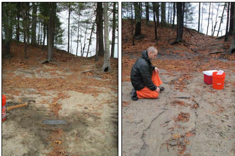
Installation of the stormwater sampler on November 26 (left) and recovery of the sampler on November 27 (right), following an overnight storm of 1.74 inches. Note the evidence of significant soil mobilization by flowing water in the photo to the right.
